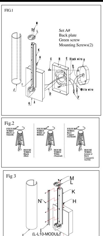
**IMPORTANT:** Fixture should be installed by a qualified electrician to ensure proper wiring and installation. Dimmable with C-L (CFL & LED) type and Incandescent/Halogen type dimmers
