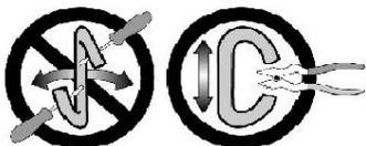
Notice: It is important to use proper chain pliers (not included) To OPEN and CLOSE the chain included with this fixture. Do not open them with other tools that may twist or stress the chain links. It is important to use proper chain pliers like the ones shown in the diagram.
