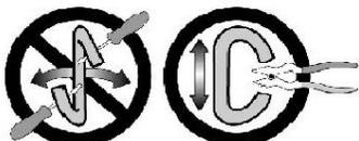
Notice: It is important to use proper chain pliers (not included) To OPEN and CLOSE the chain included with this fixture. Do not open them with other tools that may twist or stress the chain links. It is important to use proper chain pliers like the ones shown in the diagram.
