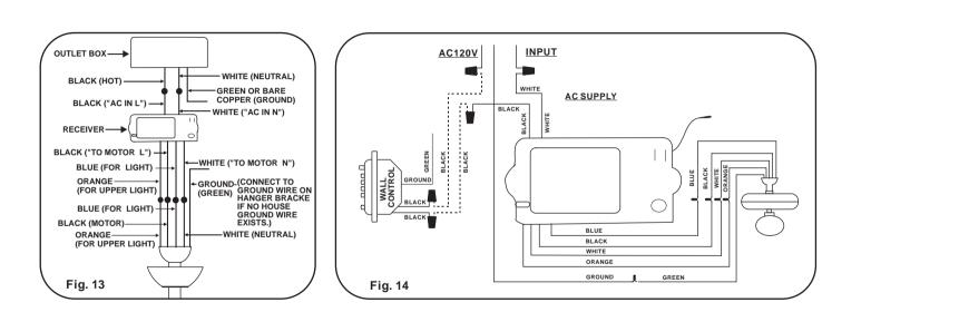
WARNING! HOOK UP "IN SERIES" ONLY. DO NOT CONNECT NEUTRAL SUPPLY WIRE OF ELECTRIC CIRCUIT TO THE TRANSMITTER WALL SWITCH, DAMAGE TO THE TRANSMITTER WALL SWITCH AND POSSIBLE FIRE COULD OCCUR.
