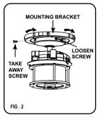
Step 3. Install the mounting bracket with provided mounting hardware A.
