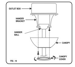
Step 1. Remove 1 of the 2 screws from the bottom of the hanger bracket and loosen the other one half a turn from the screw head.
