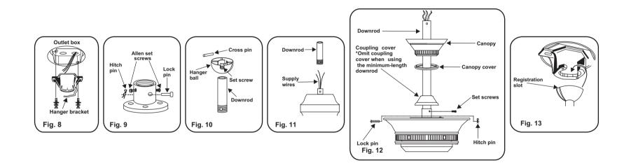
WARNING: To avoid possible electrical shock be sure electricity is turned off at the main fuse or breaker box before wiring. Step 2. Motor to Receiver Electrical Connections: Connect the WHITE wire from the fan to the WHITE wire marked "TO MOTOR N" fu
