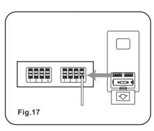
Step 2: Connect the motor plug and light plug to the receiver connector. Then, Connect the White and black wire from the outlet box to the white and black wire from the receiver.
